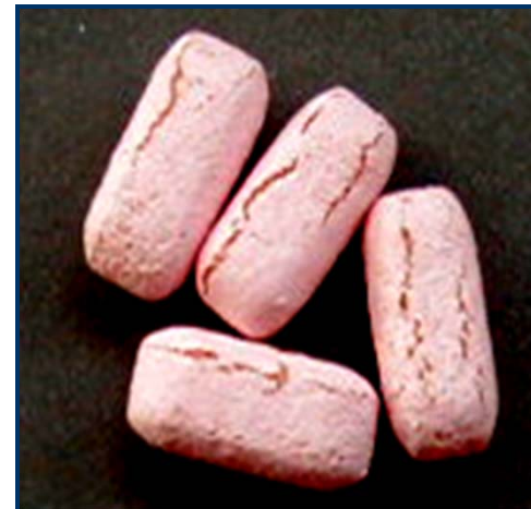
4. Tablet Swelling & Film Cracking
